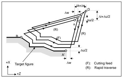
Fig. 5.8.3 (a) Cutting path in pattern repeating
