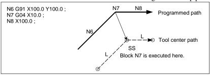
In offset mode, the number of blocks without movement consecutively specified must not exceed N-2 (where N is the number of blocks to read in offset mode (parameter No. 19625). If commanded, a vector whose length is equal to the offset value is produced in a normal direction to tool motion in earlier block, so overcutting may result.
