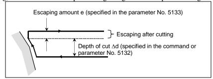
Fig. 7.1.1 (j) Cutting along the workpiece figure (type II)
