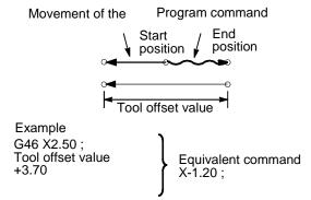
2 Tool offset can be applied to circular interpolation (G02, G03) with the G45 to G48 commands only for 1/4 and 3/4 circles using addresses I, J and K by the parameter setting, providing that the coordinate system rotation be not specified at the same time. This function is provided for compatibility with the conventional CNC program without any cutter compensation. The function should not be used when a new CNC program is prepared.
