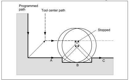
There is no actual interference, but since the direction programmed in block B is opposite to that of the path after the cutter compensation, the tool stops and an alarm is displayed.
