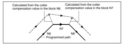
Fig. 6.4 (c) Changing the cutter compensation value
