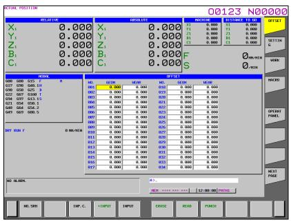
Fig. 1.1.1 (f) Tool compensation memory B (15-inch display unit)
