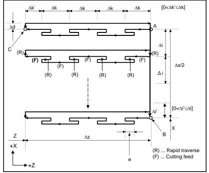
Fig. 5.8.5 (a) Cutting path in end face peek drilling cycle
