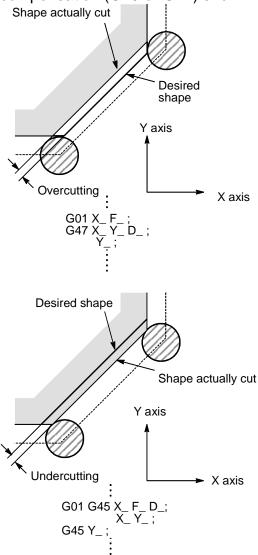
2 G45 to G48 (tool offset) must not be used in the G41 or G42 (cutter compensation) mode.
