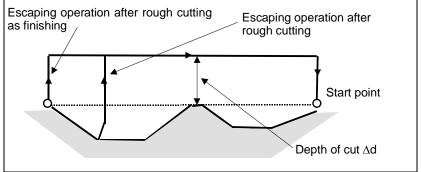
Fig. 7.1.1 (I) Escaping operation when the tool returns to the start point (type II)
