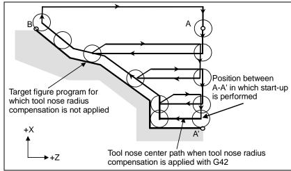
Fig. 7.1.1 (r) Path when tool nose radius compensation is applied
