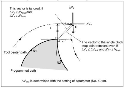
If the vectors are not judged to almost coincide (therefore, are not erased), movement to turn around the corner is performed. The corner movement that precedes the single block stop point belongs to the previous block, while the corner movement that succeeds the single block stop point belongs to the latter block.
