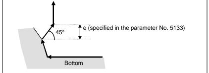
Fig. 7.1.1 (k) Escaping from the bottom to the direction of 45 degrees
