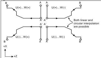
Fig. 5.8.1 (b) Four target figure patterns
