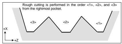
Fig. 5.8.1 (I) Rough cutting order in the case of monotone decrease (type II)
