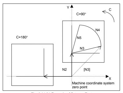
Fig. 6.14 (b) Example of fixture offset
