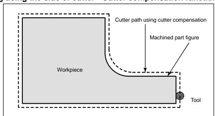
Because a cutter has a radius, the center of the cutter path goes around the workpiece with the cutter radius deviated.
