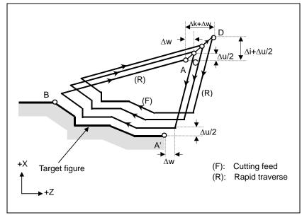
Fig. 7.1.3 (a) Cutting path in pattern repeating
