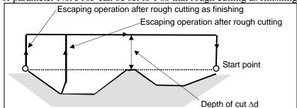
Fig. 5.8.1 (k) Escaping operation when the tool returns to the start point (type II)
