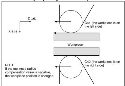
Fig. 6.5.4 (b) When the workpiece position is changed
