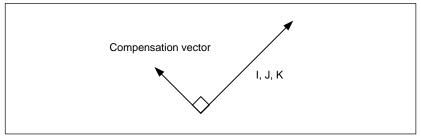
In G42 mode, the direction specified by I, J, and K is assumed an imaginary tool movement direction, and an offset vector is created vertical to that direction and on the right side.
