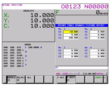
Fig. 1.1.4 (c) Fixture offset setting screen (10.4-inch display unit)
