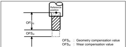
Fig. 6.10 (a) Geometric compensation and wear compensation
