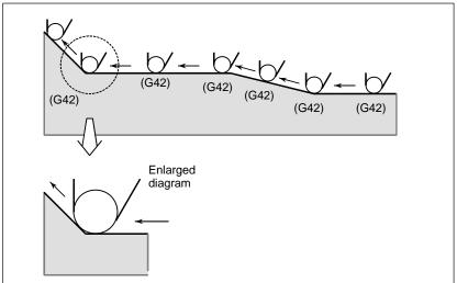
Fig. 6.5.4 (c) Tool movement when the workpiece position does not change
