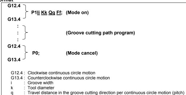
Feedrate (speed of the center of a tool that performs continuous circle motion)
