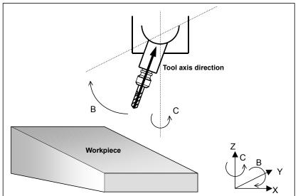
Fig. 6.15 (a) Tool Axis Direction Tool Length Compensation
