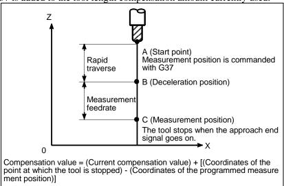
Fig. 6.2 (a) Automatic tool length measurement
