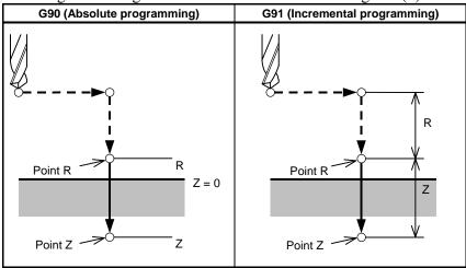
Fig. 5.1 (b) Absolute programming and incremental programming
