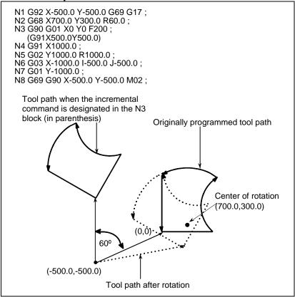
Fig. 6.11 (c) Absolute/incremental programming during coordinate system rotation
