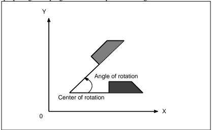
Fig. 6.11 (a) Coordinate system rotation
