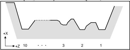
Fig. 5.8.1 (f) Figure having pockets (type II)
