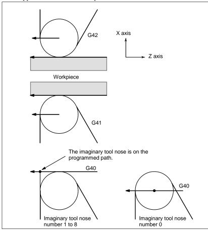
Fig. 6.5.4 (a) Workpiece position
