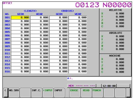
Fig. 1.1.1 (c) Tool compensation memory C (10.4-inch display unit)
