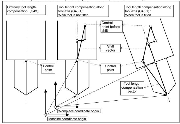
Fig. 6.15.1 (c) Shift of the Control Point
