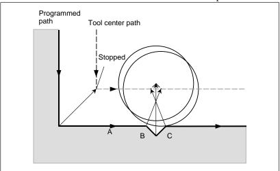
Like <1>, an alarm is displayed because of the interference as the direction is reverse in block B.
