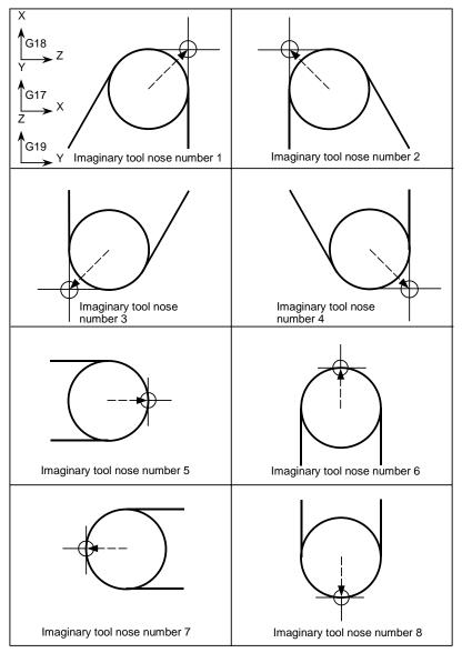
Fig. 6.5.2 (a) Direction of imaginary tool nose
