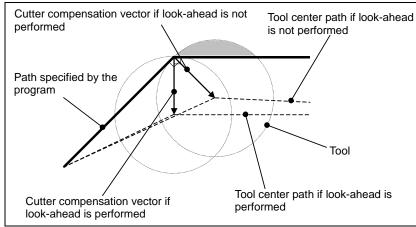
N7 contains G49 (cancellation of tool length compensation) in G42 mode and, therefore, look-ahead of N8 and subsequent blocks is not performed.
