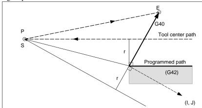
When an intersection is not obtainable, the tool comes to the normal position to the previous block at the end of the previous block.
