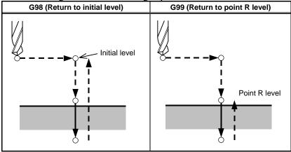
Fig. 5.1 (c) Initial level and point R level
