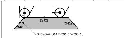
Fig. 6.5.4 (h) Specification of G41/G42 in G41/G42 mode
