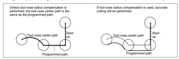
Fig. 6.5.1 (c) Tool path when programming using the tool nose center
