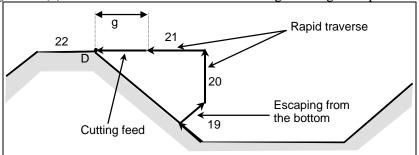
Fig. 5.8.1 (o) Details of motion after cutting for a pocket (type II)
