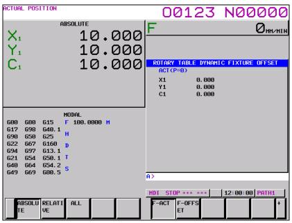
Fig. 1.1.4 (a) Active fixture offset display screen (10.4-inch display unit)
