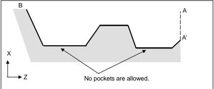
Fig. 5.8.1 (c) Figure which does not show monotone increase or decrease (type I)
