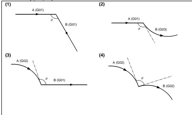
In the tool radius compensation mode as well, an automatic exact stop check is made for the corner inner angles of the programmed path. At this time, an exact stop is performed at points A and B in the figure below. (Point S represents a single-block stop point.)
