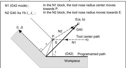
In this case, note that the CNC obtains an intersection of the tool path irrespective of whether inner or outer side machining is specified.
