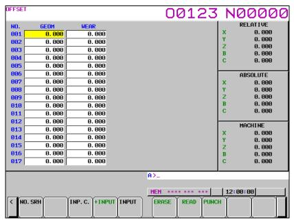
Fig. 1.1.1 (b) Tool compensation memory B (10.4-inch display unit)
