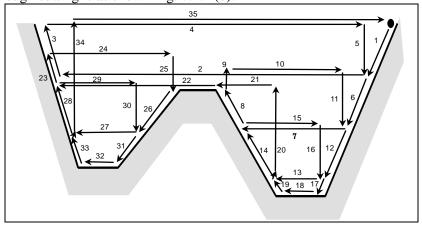
Fig. 7.1.1 (o) Cutting path for multiple pockets (type II)
