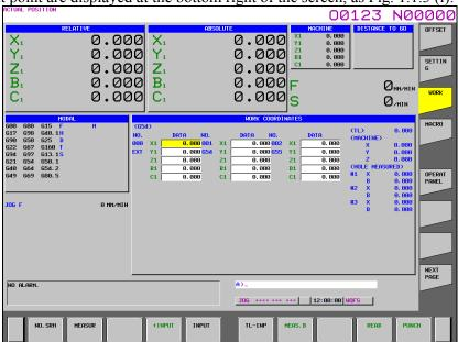
Fig. 1.1.3 (I) Workpiece origin offset setting screen (15-inch display unit)
