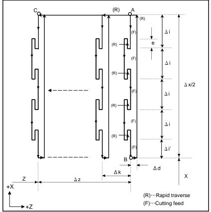
Fig. 5.8.6 (a) Outer diameter/internal diameter drilling cycle
