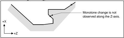
Fig. 5.8.1 (g) Figure which cannot be machined (type II)
