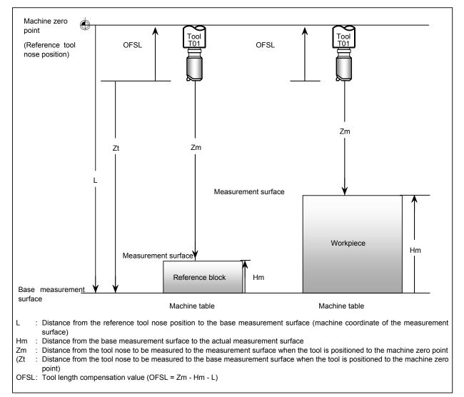
Defining the actual tool length as the tool length compensation has the advantage of eliminating the need for remeasuring, even if the workpiece is changed, provided the tool is not worn. Another advantage is that the tool length compensation need not be re-set when multiple workpieces are machined. In this case, assign a workpiece coordinate system to each workpiece, using G54 to G59, and set the workpiece origin offset for each workpiece.
