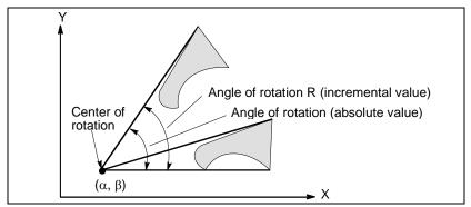
Fig. 6.11 (b) Coordinate system rotation
