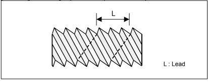
Fig. 3.4 (a) Multiple thread screws
