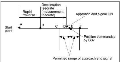
Fig. 6.2 (b) Tool movement to the measurement position
