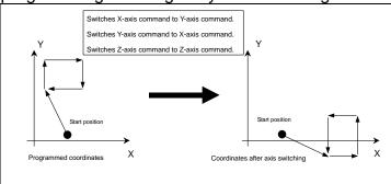
2 The hole machining axis in a canned cycle and tool length compensation and the axis to which tool length compensation is applied can be fixed at the Z-axis by setting bits 1 (TLB) and 0 (TLC) of parameter No. 5001 and bit 0 (FXY) of parameter No. 5101. Even in this case, however, if program address Z is changed to the machine axis x or y by axis switching, the hole machining axis and the axis to which tool length compensation is applied are also changed to x or y.
