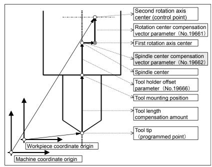
Fig. 6.15.1 (b) Spindle Center Compensation
