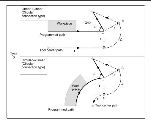
If the cancel block is a block with tool movement, and the tool moves around the outside at an acute angle of 1 degree or less in a linear → linear manner (α≤1°)
