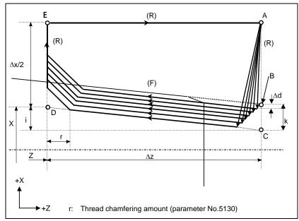
Fig. 7.1.7 (a) Cutting path in multiple threading cycle
