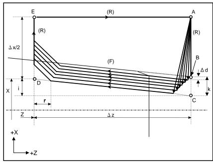
Fig. 5.8.7 (a) Cutting path in multiple threading cycle
