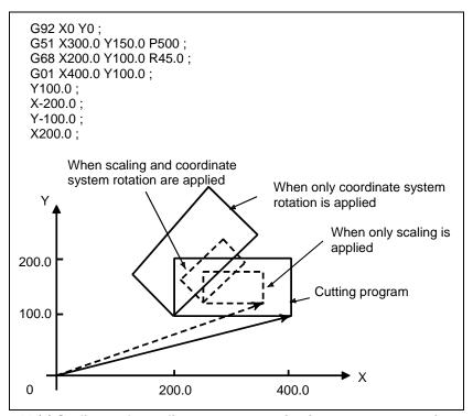
Fig. 6.11 (e) Scaling and coordinate system rotation in cutter compensation mode
