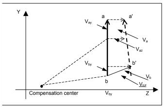
Fig. 6.12 (i) Path on the Y-Z plane
