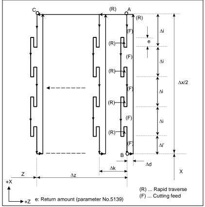
Fig. 7.1.6 (a) Outer diameter/internal diameter drilling cycle
